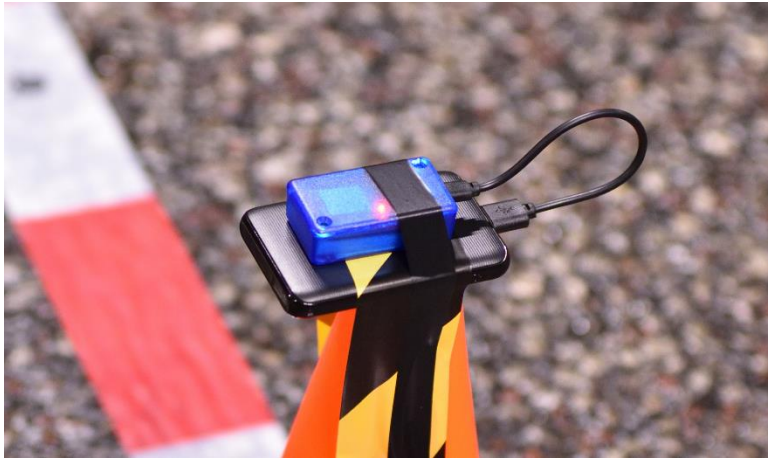
Figure 3. Wi-Fi device with battery used during the experiments to represent a mobile phone.
