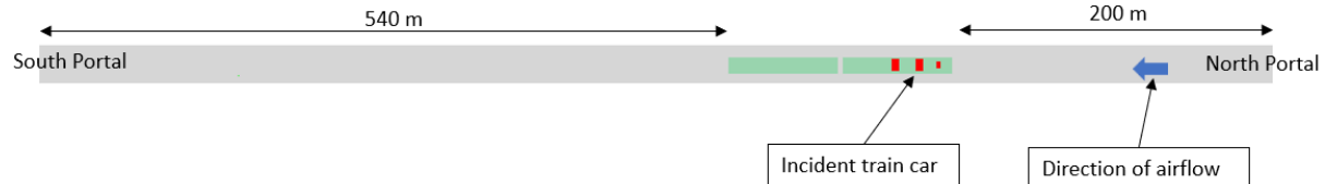
Figure 4 Fire simulation configuration
